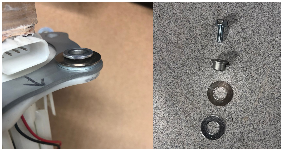
Fig. 5 (EFI Pump/Metal OEM Flange-Ring/IMS Flat Washer/OEM Crush Washer/OEM Sleeve Combo)
